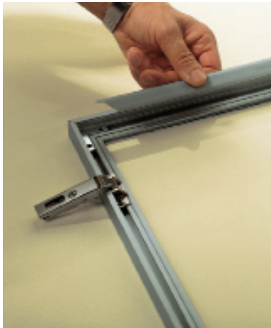
7) Cut to length and mitre the internal frame over profile also.
