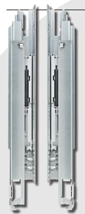
DYNAPRO Soft-close undermount slides are available in 9", 12", 15", 18", 21", 24", 27" & 30" lengths. The slide is suitable for drawer material of 1/2" to 5/8", as well as a version for 3/4" drawer material. You have the option of a 2D slide offering height and side adjustment, or a 3D slide offering height, side and rear tilt adjustment. Dynapro is available with a standard dynamic load rating of 88 pounds or a heavy duty dynamic load rating of 132 pounds.
